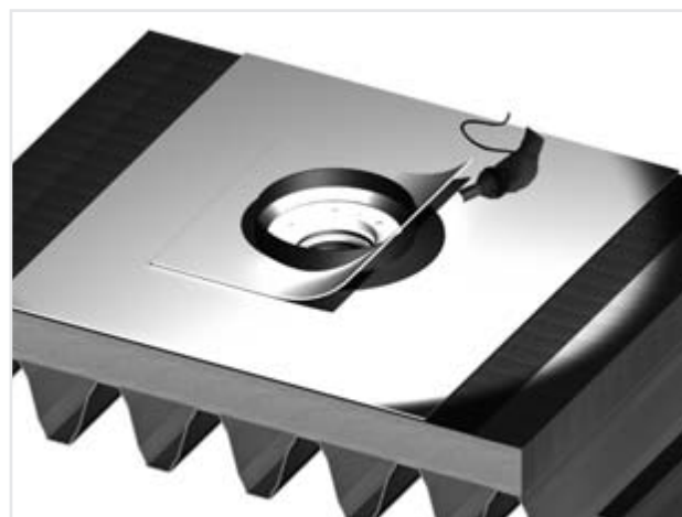
Figure 12.36 Placement de la manchette PVC
